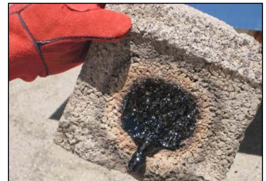
Cinder Block after two minutes in beam
